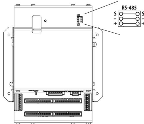
4. Mechanically secure the RS-485 cable(s) where it/they enter the electrical panel.
