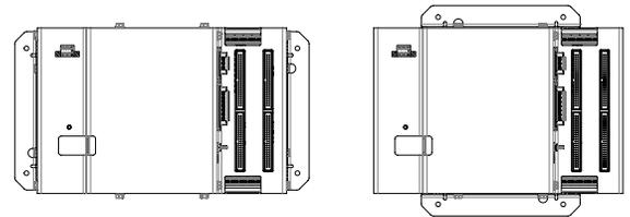
Install the E30E in the panel (hardware not provided). A grounding connection is located on the housing (see below).
