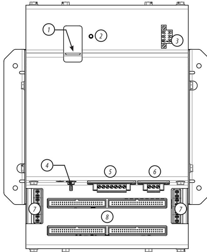
1. Ethernet Port: Provides Ethernet connection for the gateway component.
