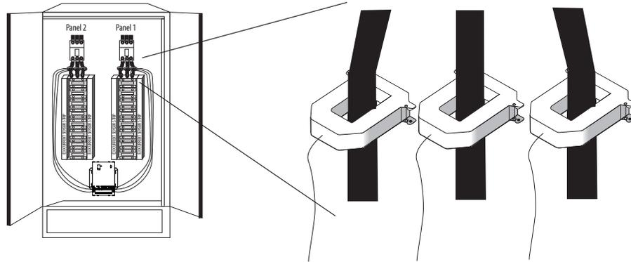
Note: The E30E measures and reports the phase angle of each voltage input and each CT (when there is active current through the primary of that CT). Use the NetConfig configuration software tool to view the phase angles of active circuits to help verify that those circuits are connected to and mapped to the proper voltage phases. See the E3x Commissioning Guide ([www.veris.com](http://www.veris.com)) for instructions on how to download and operate the tool from a PC.
