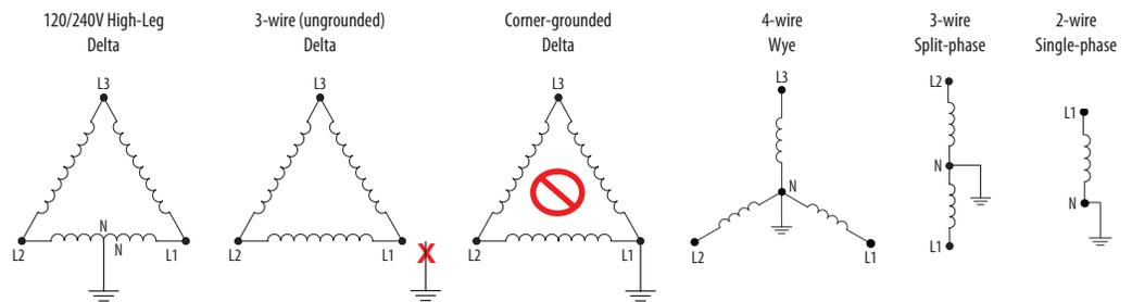
120 V/240 V Delta High Leg (where the center tap of one of the three phase-to-phase transformers is grounded): the E3x supports these applications, as long as the line-to neutral voltage [especially of the High Leg] does not exceed 300 Vac (as in North American 120/240 V High Leg Delta configurations).
