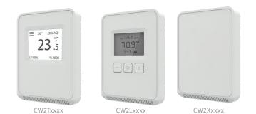
The CW2 Series of air quality sensors for living space is a flexible multi-sensor platform for use with BAS controllers designed to accept 4 to 20mA, 0 to 5Vdc or 0 to 10Vdc outputs. CW2 Series sensors are available with three user interface options: touchscreen, LCD with three buttons and blank.  $CO_2$  and temperature sensors are included with all CW2 Series air quality sensors. Models with VOC sensors and relative humidity sensors are also available.
